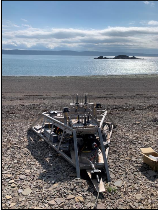
Figure 11: The cabled subsea platform developed for the VITALITY project just prior to deployment in the intertidal zone.
