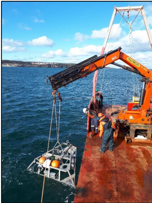
Figure 4: Deployment of the FAST platform in Grand Passage for an assessment of PAM instrument performance.
