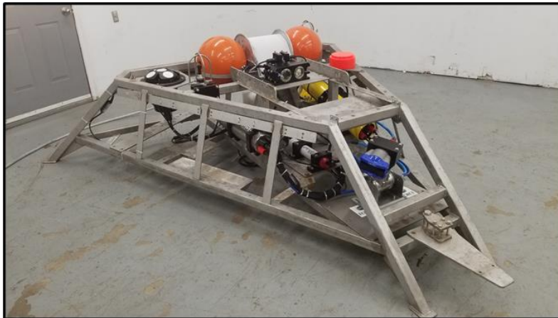
Figure 5: The integrated sensor platform developed by DP Energy under the Pathway Program.
